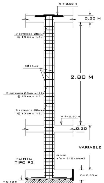
DETALLE DE COLUMNA Y PLINTO ARMADURA
